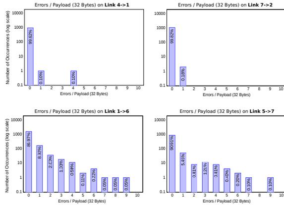
Fig. 11: Error Patterns: *Strong* Links (top) and *Weak* Links (bottom)
