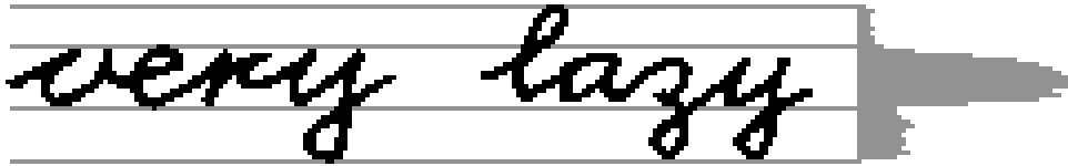
Figure 1: An example of binarization, horizontal projection profile computation, and reference line extraction.
