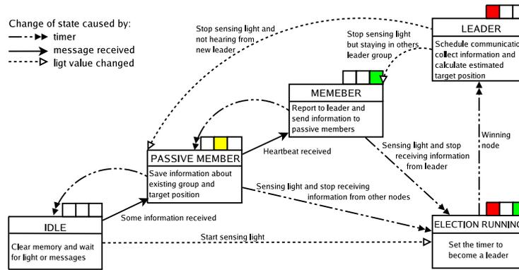
Fig. 5: State diagram for ESB implementation of the DELTA node's roles.
