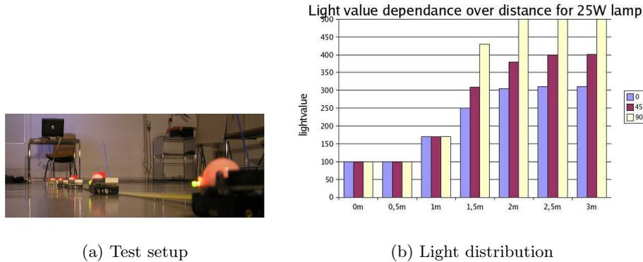
Fig. 1: Light distribution test setup and results.
