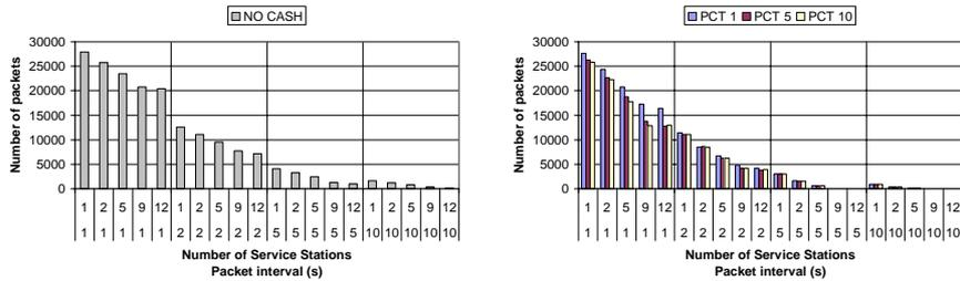
**Fig. 14.** Number of dropped packets due lack of Traffic Credits of the old and the improved CASHnet scheme for different packet counter thresholds, PCT.
