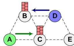
**Fig. 6.** Without cooperation only single-hop connections are possible and the network falls apart.
