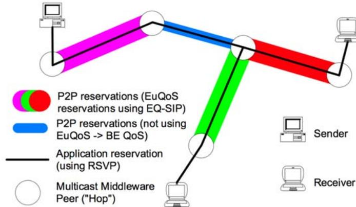
**Fig. 2.** QoS Reservations using BE-QoS or EuQoS-Signaling
