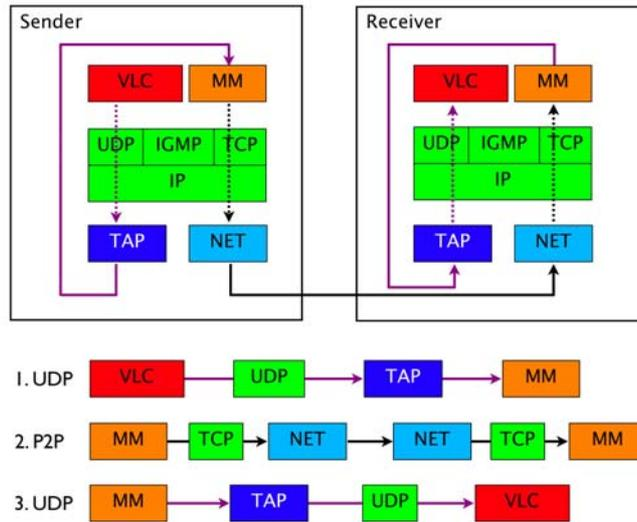
**Fig. 4.** Sender controlled Broadcasting of UDP Multicast Traffic
