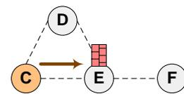
**Fig. 9.** E does not forward C's packets destined for F
