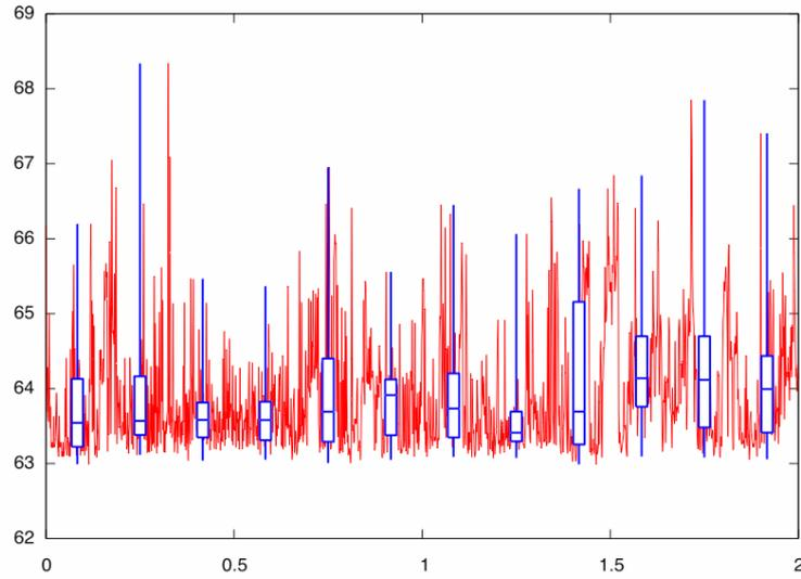
**Fig. 1.** A time series of round trip times, and the corresponding percentile vectors.
