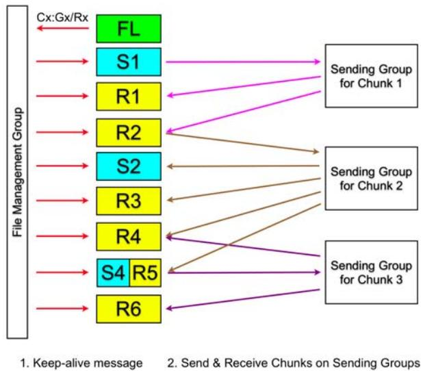
**Fig. 3.** Sending and receiving of chunks
