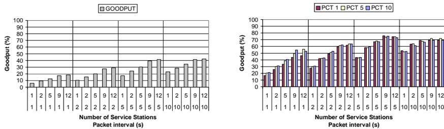
**Fig. 13.** Goodput of the old and the improved CASHnet scheme for different packet counter thresholds, PCT.
