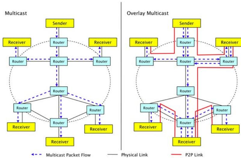
**Fig. 1.** Traditional Multicast vs. Overlay Multicast
