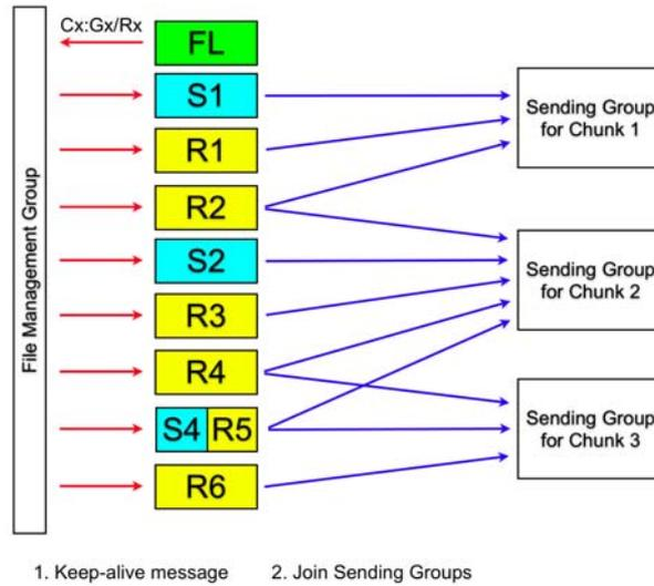
**Fig. 2.** Joining of senders and receivers to the chunk sending groups
