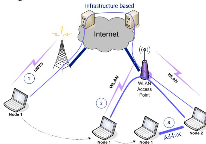
**Fig. 1.** Seamless Switching between Infrastructure and Ad-hoc Mode
