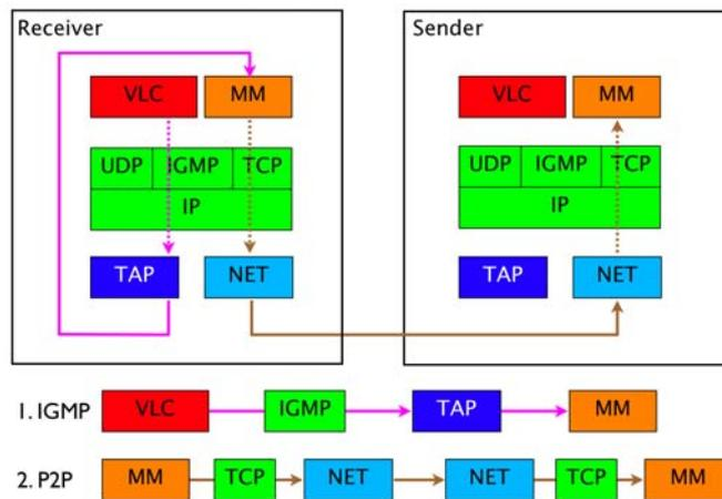
**Fig. 3.** Receiver initiated Multicast Group join
