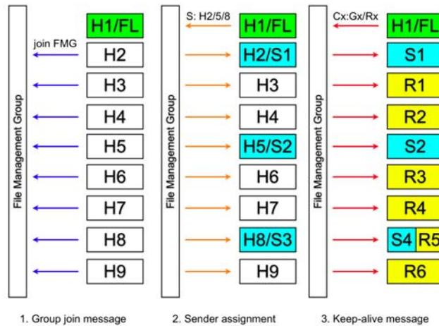
**Fig. 1.** Host joining, sender assignment and keep-alive message sending
